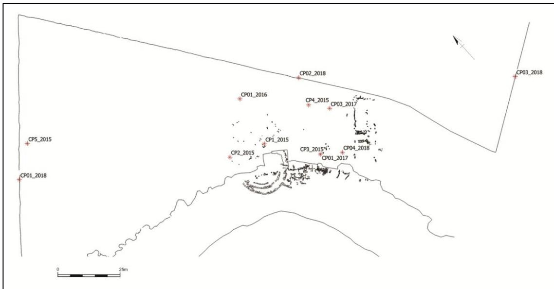
Figure 4: Plan of the site showing the location of the survey control points.
